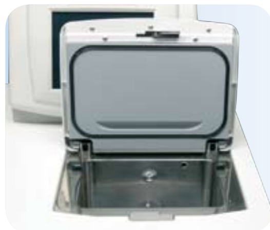
Internal heated retort lid and condenser
